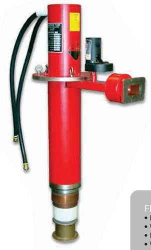
CPI Microwave Power Products (MPP) offers the VKS-8262 series of klystrons for use in particle accelerators for scientific, medical, and industrial applications. These klystrons provide up to 7.5 MW peak at 2.856 or 2.9985 GHz at various rf pulse lengths and duty. Versions are available with up to 36 kW of average output power at 2.856 GHz and 72 kW at 2.9985 GHz.
